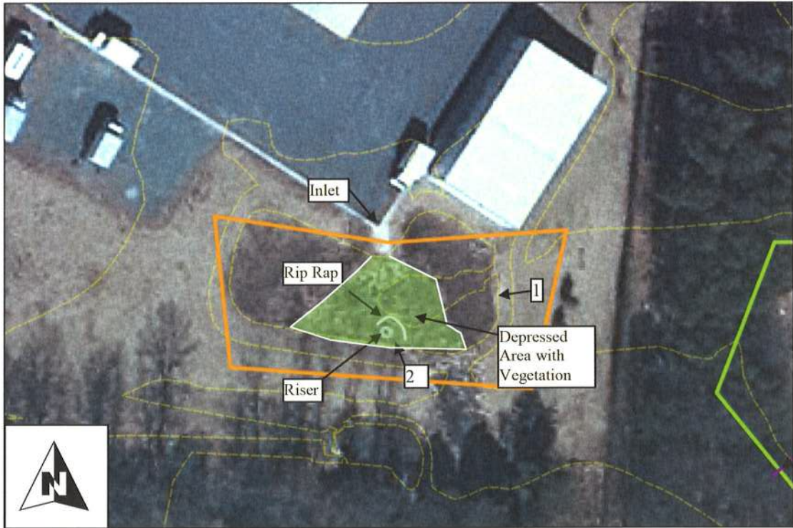
Existing Condition: Facility has broken low flow orifice and is in need of maintenance.
