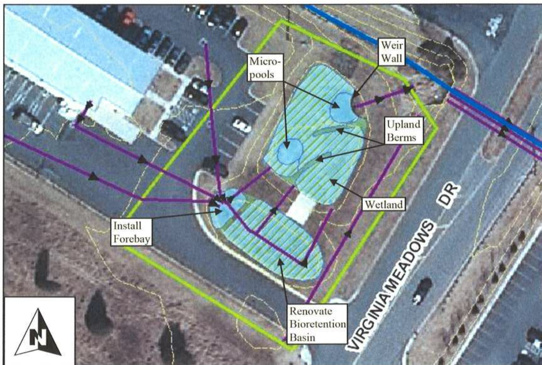
Conceptual Plan: Renovate bioretention basin and install forebay to capture sediment. Improvements to dry basin including micro-pools, wetlands, berms and weir wall outlet structure
