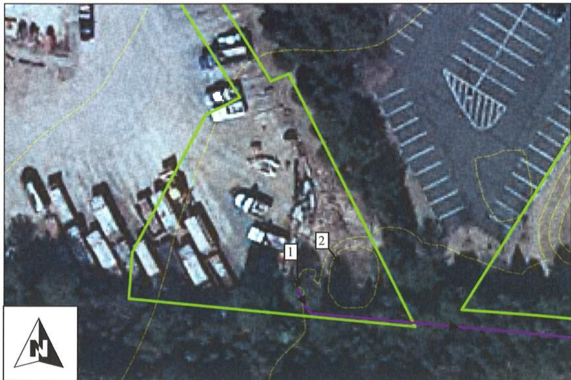
Existing Condition: BMP is not maintained, and parking has encroached into easement
