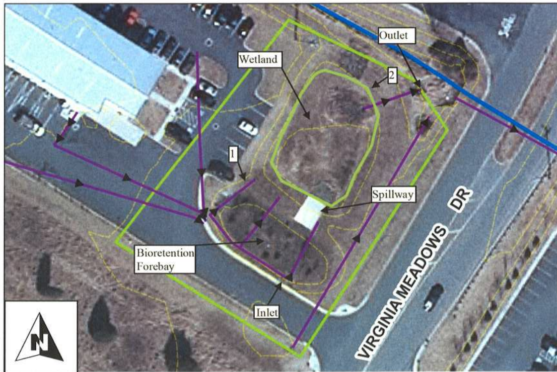
Existing Condition: Site with bioretention forebay and dry basin without riser
