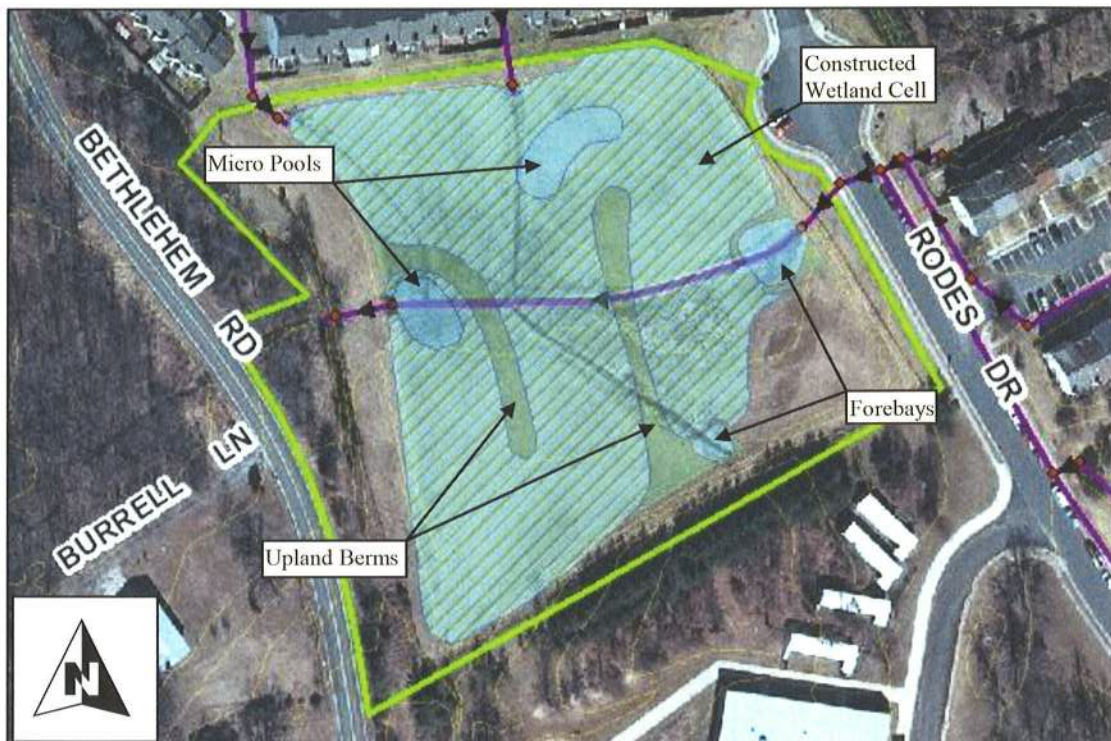
Conceptual Plan: Constructed stormwater wetland with forebays for pre-treatment and upland berms to increase flow lengths and residence time
