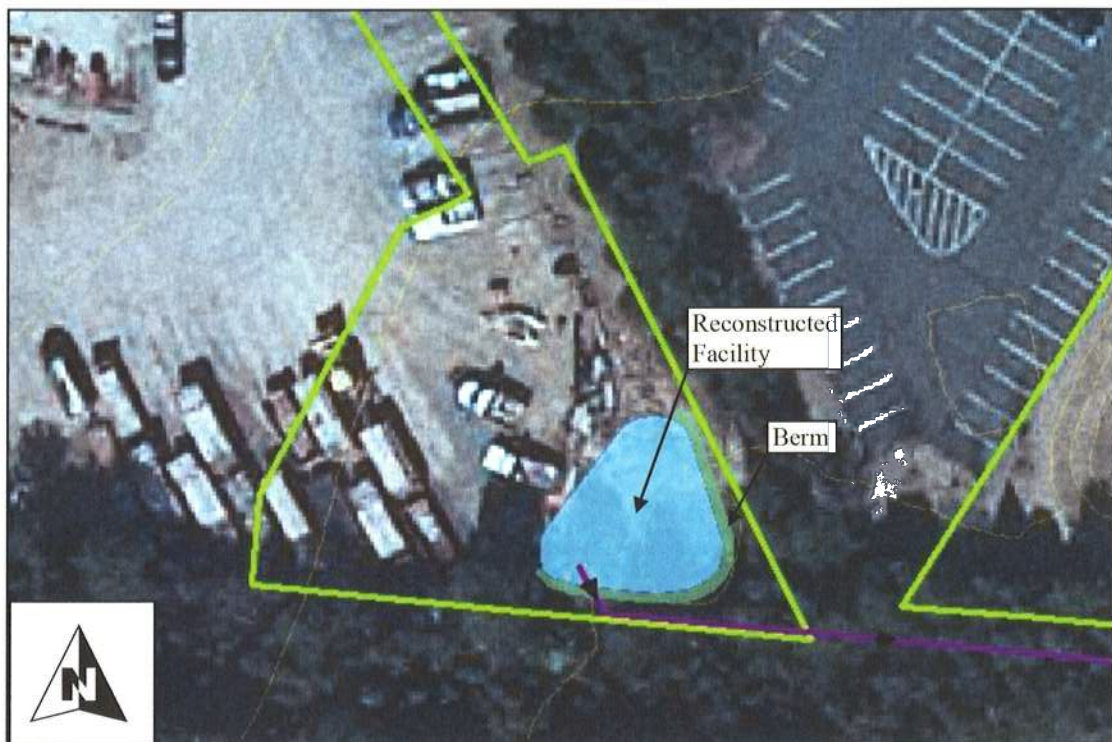
Conceptual Plan: Reconstructed detention facility with minimum footprint.
