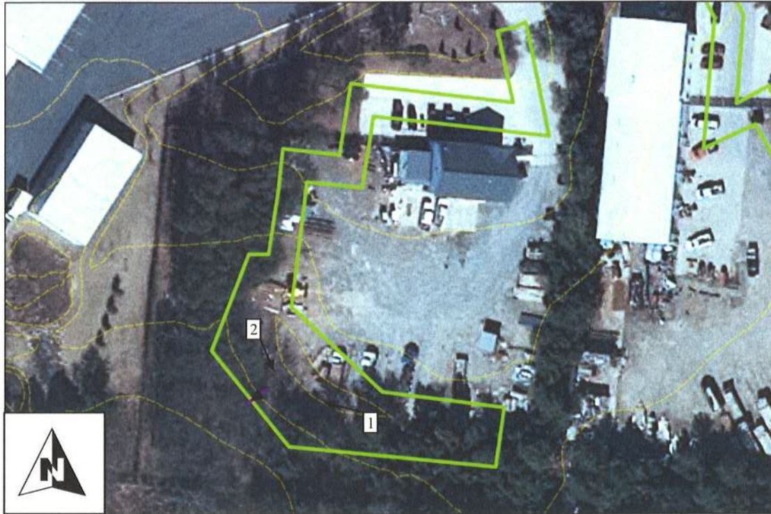
Existing Condition: SWMP/BMP has been impacted by expansion of parking area
